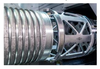
View into the machine: The fine boring tool from MAPAL for high-precision external machining of the thin-walled pot-shaped stator housings. ©MAPAL
