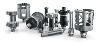
MAPAL presents tool solutions for the complete machining the pot-shaped stator housing on machining centres. ©MAPAL
